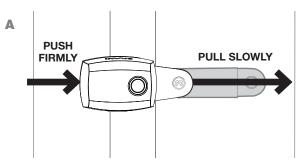
After tab 3 has been removed, press lock against front panel for 10 seconds to set adhesive.
