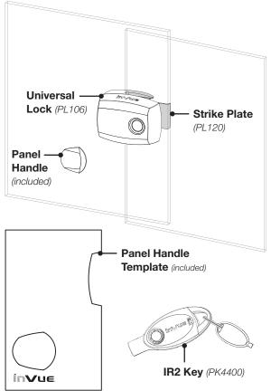
Determine if the front panel is on the left or right hand side. Note: The illustrations in this booklet are for right front panel orientation. For left front panel cabinet install in opposite direction.
