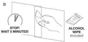
IMPORTANT! Allow alcohol to air dry for a minimum of 5 minutes or dry alcohol with lint free cloth before moving to step 2.
