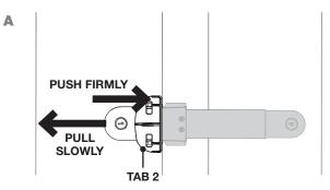
Press tab 2 towards back panel and hold for 10 seconds.
