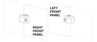
Wipe front and back of both panel surfaces with alcohol wipe where you intend to mount the lock.
