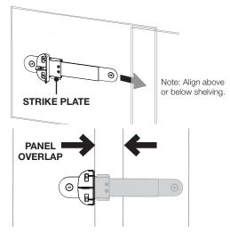
Note: Strike Plate size is determined by width of panel overlap.
