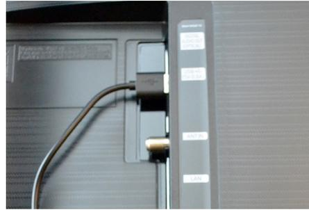
2 Plug the USB end of the micro USB/USB-A power cable (included in the DBD705 Interface Cable kit).
