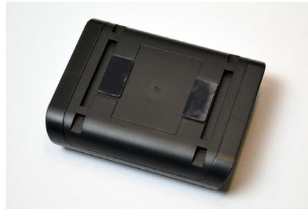
6 If mounting the sensor using the provided adhesives, remove the adhesives from their backing and place it into the flat area on the bottom of the sensor.
