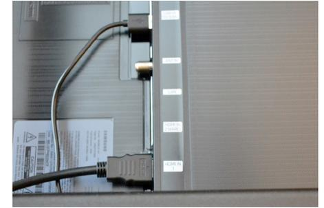
4 Plug an HDMI cable into HDMI port 1 on the TV.
