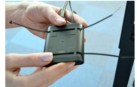
8 If mounting the sensor using the provided zip ties, loop the zip ties through the slots on the back of the TV Sensor.
