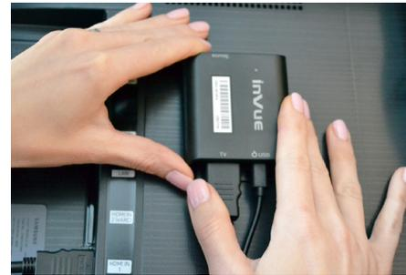
7 Peel the clear film from the adhesives. Place the TV Sensor on a flat surface and apply pressure for at least 10 seconds.
