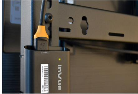
10 If running content through the TV Sensor, plug another HDMI cable into the port on the sensor marked "Source". Connect the other end to your Content Management System.
