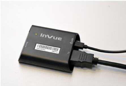
5 Plug the other end into the port marked "TV" on the sensor.
