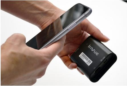
1 Within the InVue LIVE app, use the camera on your device to scan the code and enroll the sensor. Fill out the information for the sensor and the device that will be displayed.
