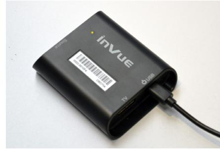
3 Plug the micro USB end of the power cable into the port on the sensor. With the TV powered on, allow the sensor to charge for 5 hours. This will need to be done every time the battery in the sensor is depleted.
