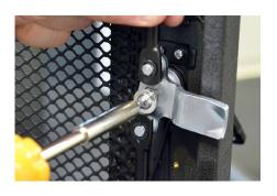
Secure the shaft with the provided screw.
