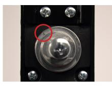
Determine which way the handle will turn. With the shaft adapter in the position above, the handle will turn to the right.
