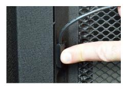
Place the sensor where previously determined and apply pressure for at least 10 seconds.
