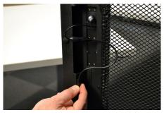
Do NOT place the sensor where the cable will bunch up and prevent the door from opening and closing easily.
