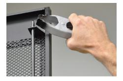
Remove the clamp from the swing bar.
