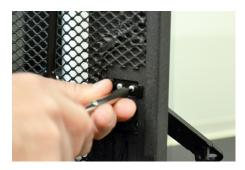
Align one of the brackets with the top screw inserts. Insert and tighten 2 of the screws to secure the bracket.
