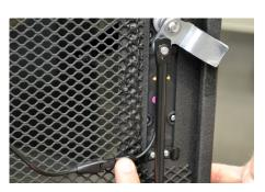
Position the cable so that it will be out of the way or the cam arm's action. Press the adhesive against the surface for at least 10 seconds.
