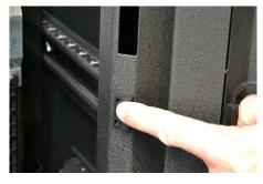
Place the sensor where previously determined so that it will sit in range of the other magnet sensor when the door is closed. Apply pressure for at least 10 seconds.
