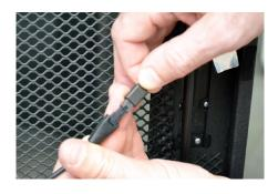
Plug the sensor cable into the cable on the back of the RAC Lock.
