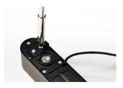
Remove the 2 screws holding the top bracket on the back of the RAC Lock body.
