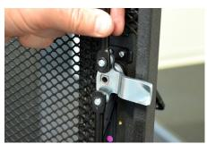
Place the cam arm onto the shaft.
