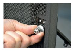
Place as many spacers onto the shaft to still allow room for the cam arm.
