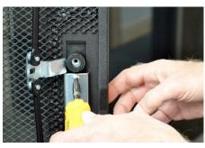
Position the cam arm and swing bar to the side. Remove the hardware and panel holding the old lock to the door.
