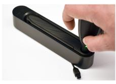
Place an installer OneKEY into the IR port on the lock and press the button on the key.
