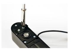
Remove the 2 screws holding the top bracket on the back of the RAC Lock body.
