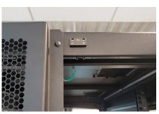
Remove the clear film from the other independent magnet sensors and place it at the top of the door frame so that it will align with the top sensor bracket sensor. Apply pressure for at least 10 seconds.
