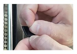
**Optional:** If there is excess sensor cable that may get caught, remove the backing from the adhesive on the provided cable anchor.
