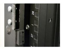
Peel the clear film from the adhesive on the independent magnet sensor. Place it below the latch in the door frame as shown. Apply pressure for at least 10 seconds.
