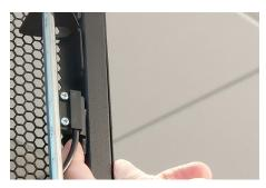
Place the secondary bracket on the inside of the door panel, below the bracket that holds the swing bar. Apply pressure for at least 10 seconds.
