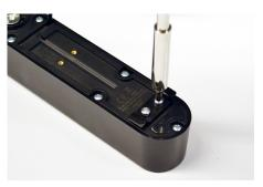
Remove the 2 screws holding the bottom bracket on the back of the RAC Lock body.
