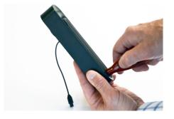
Place an installer OneKEY into the IR port on the lock and press the button on the key.
