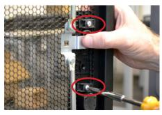
Position the cam arm and swing bar to the side. Remove the screws and brackets holding the old lock to the door.
