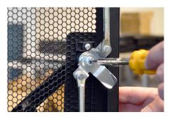
Remove screw holding the cam arm to the old lock.
