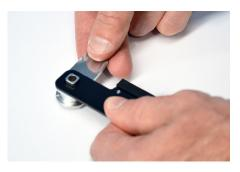
Place the sensor arm over the cam arm.
