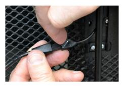
Peel the clear film from the adhesive on the RAC Lock cable.
