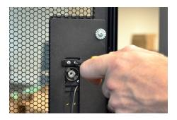
Align one of the brackets with the top screw inserts. Insert and tighten 2 of the screws to secure the bracket.
