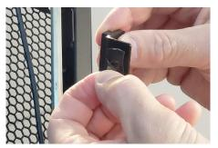
Peel the clear film from the secondary door sensor.
