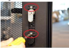
Remove the 2 screws and brackets holding the existing lock to the door.
