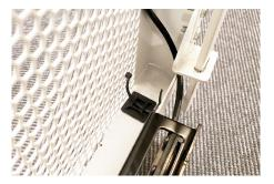
Place the cable manager in the cleaned area near the bottom sensor bracket. Apply pressure for at least 10 seconds.
