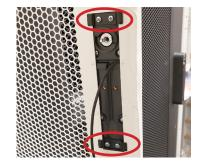
Align one of the brackets with the top screw inserts. Tighten the 2 screws to secure the bracket. Repeat for the bottom bracket.
