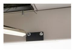
Align the template with the latch hole at the top of the rack.
