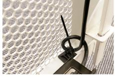
Loop the excess cable and secure it with the zip tie.
