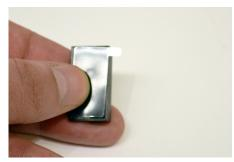
Remove one of the adhesives from its backing and place it onto the independent sensor. Press the adhesive onto the sensor for at least 10 seconds.
