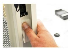
Use the provided alcohol wipe to clean the area beneath the Rac Lock. Allow it to dry completely.
