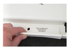
Peel the clear film from the adhesive on the independent sensor.
