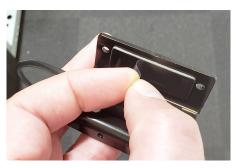
Peel the clear film from the adhesive on the bottom bracket.
