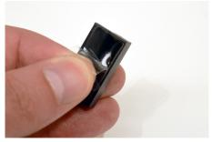
Peel the clear film from the adhesive on the independent sensor.
