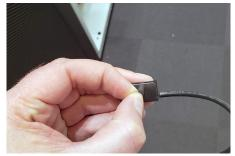
Peel the clear film from the 3rd sensor.
