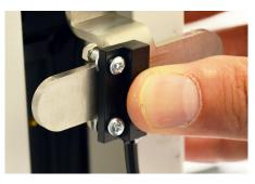
Slide the sensor onto the left side of the cam arm.
