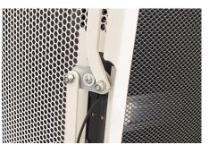
Insert and tighten the screw to secure the lock bar bracket to the lock adapter.
