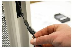
Connect the sensor cable to the Rac Lock cable.
