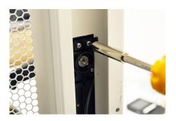
Align one of the brackets with the top screw inserts. Tighten the 2 screws to secure the bracket.
