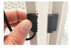
Place the sensor as shown so that it aligns with the sensor on the other door. Apply pressure for at least 10 seconds.
