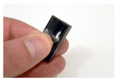
Peel the clear film from the adhesive on the independent sensor.
