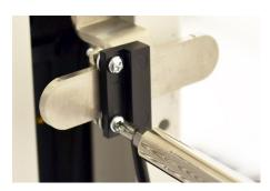
Slide the sensor onto the left side of the cam arm. Tighten the screws into the nuts to secure the sensor on the cam arm.
