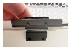
Close the door and align the bottom bracket with the bottom sensor. Apply pressure for at least 10 seconds.
