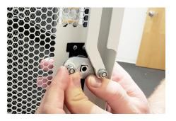
Place the lock bar bracket onto the lock adapter. The lock bar should be installed in the open position, as shown.
