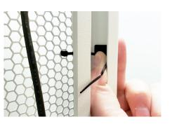
Place the cable manager in the cleaned area between the Rac Lock and the bottom of the door. Apply pressure for at least 10 seconds.
