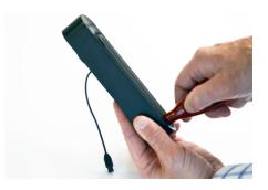
Place an installer OneKEY into the IR port on the lock and press the button on the key.
