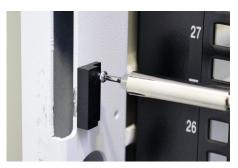
Align the holes on the sensor to the pilot holes. Secure the sensor to the frame using the included self tapping screws.
