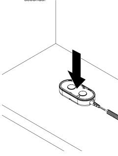
Insert one side of the pad into the rim of the base. The tabs on the pad will fit into the slots on the inner rim of the base.
