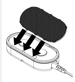
Apply pressure around the edge of the pad to fully secure the pad in the rim of the base.
