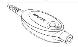
To activate the Detacher, hold a charged and coded OneKEY close to the nose of the Detacher key. Press the button on the OneKEY. The LED on the Detacher key will turn blue when successfully coded.
