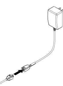
Plug the power supply into a power outlet. The LED on the key will be red.
