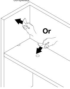
Decide how the power cable will be routed. There are 4 options; the power cable can be routed out from the back of the base (Option A), out either side of the base (Options B or C) or the power cable can be routed straight down through the fixture (Option D shown in the next step).
