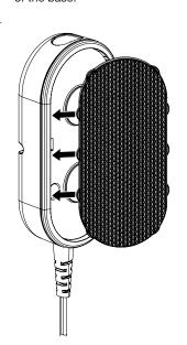
Apply pressure around the edge of the pad to fully secure the pad in the rim of the base.
