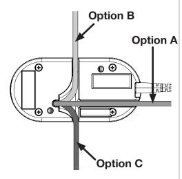
If mounting the base over a hole, the power cable can be routed straight down through the fixture.
