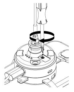
Remove the sensor and device from the stand. Place the magnet key (DBG400 or DBG406) into the depression on the sensor and push it inward to release the sensor cable. Pull the cable free.
