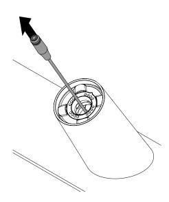
Plug the sensor cable into the sensor.
