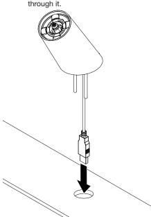
From beneath the fixture, place the metal plate over the studs and secure in place with the 2 lock nuts. Tighten fully using a 7mm deepwell socket.
