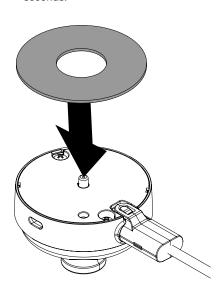
6 Plug the power connector into the device.
