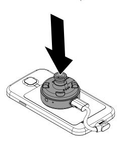
19 Attaching the Sensor to the Stand:
