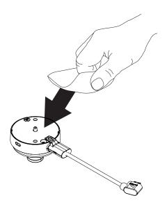
Remove the adhesive from the paper backing and place it onto the sensor. Apply pressure for at least 10 seconds.
