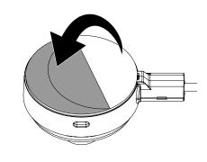
Center the sensor on the back of the device and apply pressure for at least 10 seconds.
