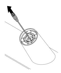
Plug the sensor cable into the sensor.
