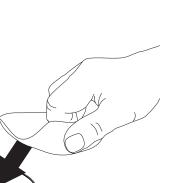
Remove the replacement adhesive (ADH2174 - Sensor replacement PSA) from the backing and place on the bottom of the alarm side. Apply pressure for at least 10 seconds.
